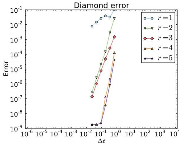
FIG. 8. The error of the diamond scheme with varying  $r$  applied to the multisymplectic Hamiltonian PDE arising from the Sine–Gordon equation. The true solution was the so-called breather on the domain  $[-30, 30]$ . The Courant number is fixed at  $\frac{1}{2}$  as  $\Delta t$  is decreased. The order of the method appears to be  $r$  when  $r$  odd and  $r + 1$  when  $r$  even (see text).
