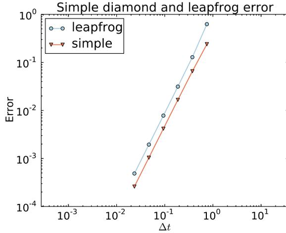
FIG. 3. The error of the simple diamond scheme applied to the multisymplectic Hamiltonian PDE arising from the Sine-Gordon equation, and the error of the leapfrog scheme applied to the Sine-Gordon equation. The exact solution is the so-called breather on the domain  $[-30, 30]$ . The Courant number is fixed at  $\frac{1}{2}$  as  $\Delta t$  is decreased. Both methods appear to have order 2.
