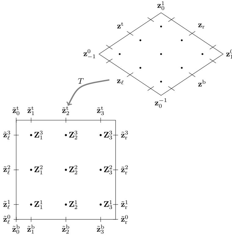
FIG. 6. The diamond transformed by a linear transformation,  $T$ , to the unit square. The square contains  $r \times r$  ( $r = 3$  in this example) internal stages,  $\mathbf{Z}_i^j$ . The solution is known along the bottom and left-hand sides. The method proceeds as two sets of  $r$  Gauss Runge–Kutta  $r$ -step methods: internal stage values,  $\mathbf{Z}_i^j, \mathbf{X}_i^j, \mathbf{T}_i^j$ , are calculated, then the right and top are updated.
