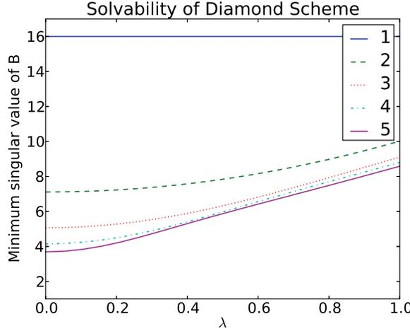
FIG. 7. How the minimum singular value of  $B$  varies with different Courant numbers. Because there are no zero singular values, the diamond scheme is solvable for the wave equation for all  $\lambda \in [0, 1]$  and  $r$  up to 5. It is easy to check this holds for larger  $r$ .
